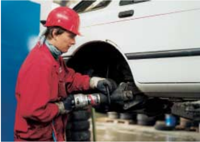
Fahrzeugrecycling z. B. Hinterachsdemontage Car recycling e.g. dismantling of the rear axle
